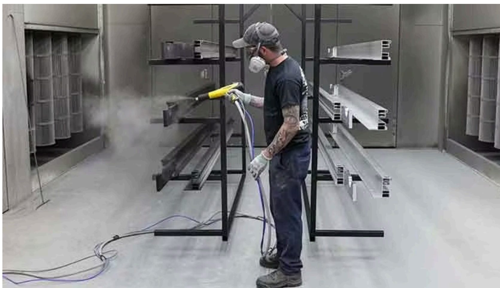
POWDER COATING BOOTH - CLOSE BOOTH FOR LARGE SIZE COMPONENTS
